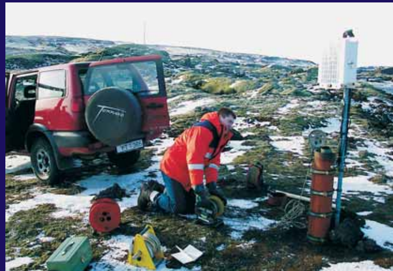
Monitoring of groundwater temperature in a borehole in Skaftártunga
