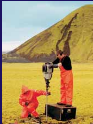
Penetration drilling at Langisjör Photo: Almenna
